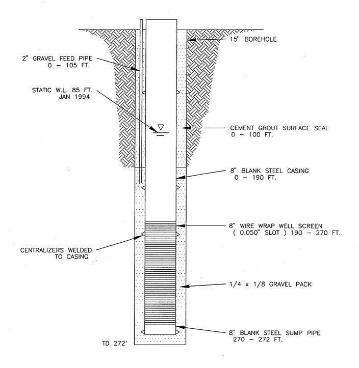
Figure 2. Production Well Construction Diagram
